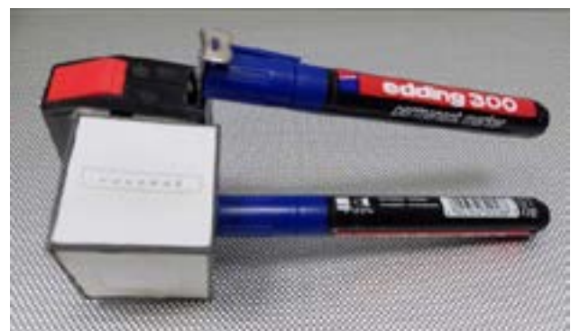
Fig. 2. Structure of the proximeter: a plastic cube, a tape-measure, and markers used as handles
