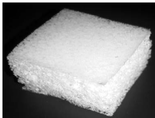
Fig. 1. Photograph of cross-linked polyvinyl formal hydrogel.
